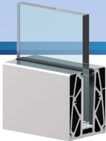
panorama XK10, you can use 8+8 mm or 10+10 mm glass panels at this system. The main difference of this system from X10 is that the glass panels are fixed with hard plastic wedges. With this characteristic it is the most economic and the most preferable system of this range.
