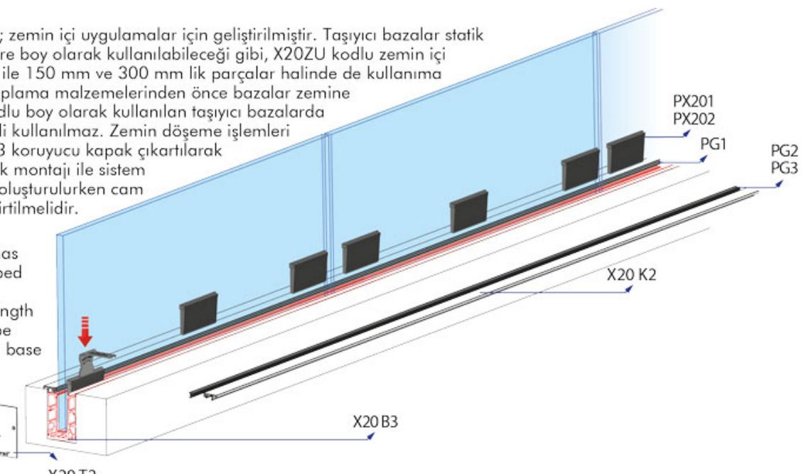
In both cases the supporting shoe is fixed to the floor before the leveling concrete and the covering material. The closer profile is applied to keep the glass groove clean. After the floor covering is finished the cover is removed and the glass panels are fixed with hard plastic wedges. The system is finished with the cladding profiles.
