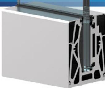
panorama XV10, the biggest benefit of using this system is the ability of aligning the glass panels upto  $\pm 2^\circ$  by fixing a set screw from the internal side. This ability helps a lot in projects where no handrail will be used on top of the glass. The system can be finished with one of the oval and straight cladding profiles upon your choice.
