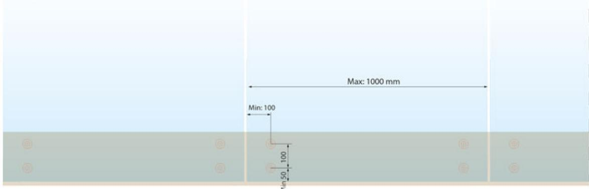
Cam delme çapı / Glass drilling diameter : Ø20 mm
