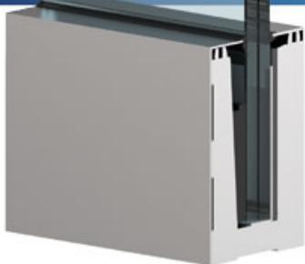
**panorama X21** is designed to resist heavy loads. The massive rail is used continuous and is suitable to install 10+10 mm or 12+12 mm glass panels up to 1200 mm height.
