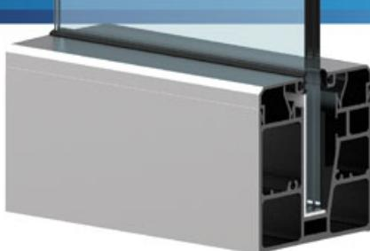
panorama S20; it is designed to resist lower loads and to be used only as continuous base shoe. The usage of a suitable handrail profile is highly recommended.
